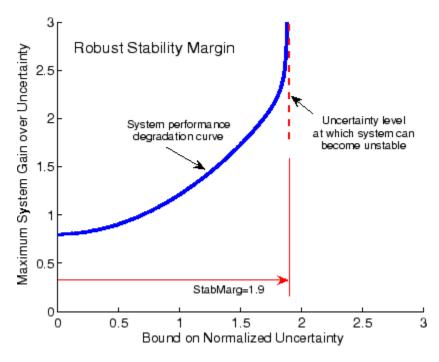
System instability is equivalent to the system gain becoming arbitrarily large, and hence characterized by the vertical line tangent to the asymptotic behavior of the performance degradation curve.
